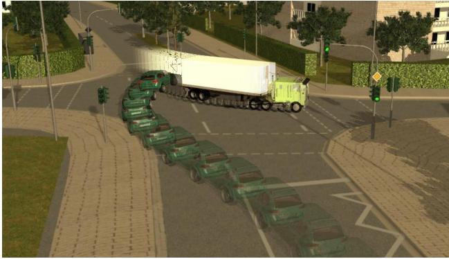
Fig. 2: Trajectory of a possible evasion maneuver performed by the car’s Digital Twin in simulation.
