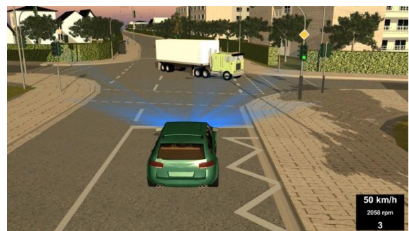
Fig. 1: Simulated scene with Digital Twins of multiple vehicles. A self-driving car approaches an intersection with oncoming traffic. The truck is about to make a left turn.
