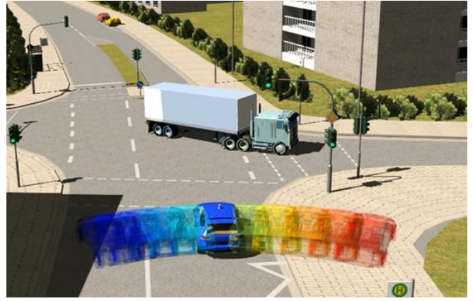
Fig. 5: “Variant ghosts” of Digital Twins. Shown are states \underline{s}(j, t') \forall j , i.e. all possible variants j for fixed time t' superimposed in one 3D scene.
