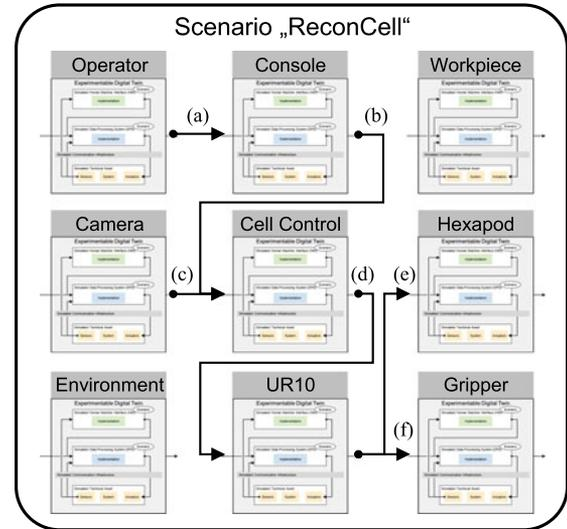
Fig. 6. Multiple interconnected and interacting EDTs make up an application scenario. Signal contents: a) operator interaction, b) op. commands, c) camera images, d) movement & gripper commands, e) fix/release, and f) open/close.
