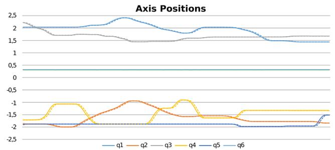
Fig. 14. Actual sampled UR10 positions during a reconfiguration process in ReconCell (solid: commanded, dashed: measured).
