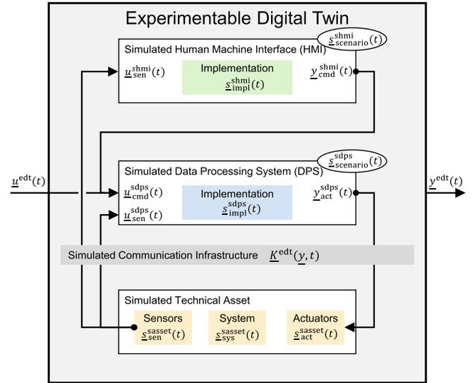
Fig. 5. Basic structure of EDTs.
