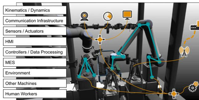
Fig. 1. Example for a “system of systems” in the field of production technology, the ReconCell [1]. Various aspects have to be investigated and integrated in comprehensive simulations.
