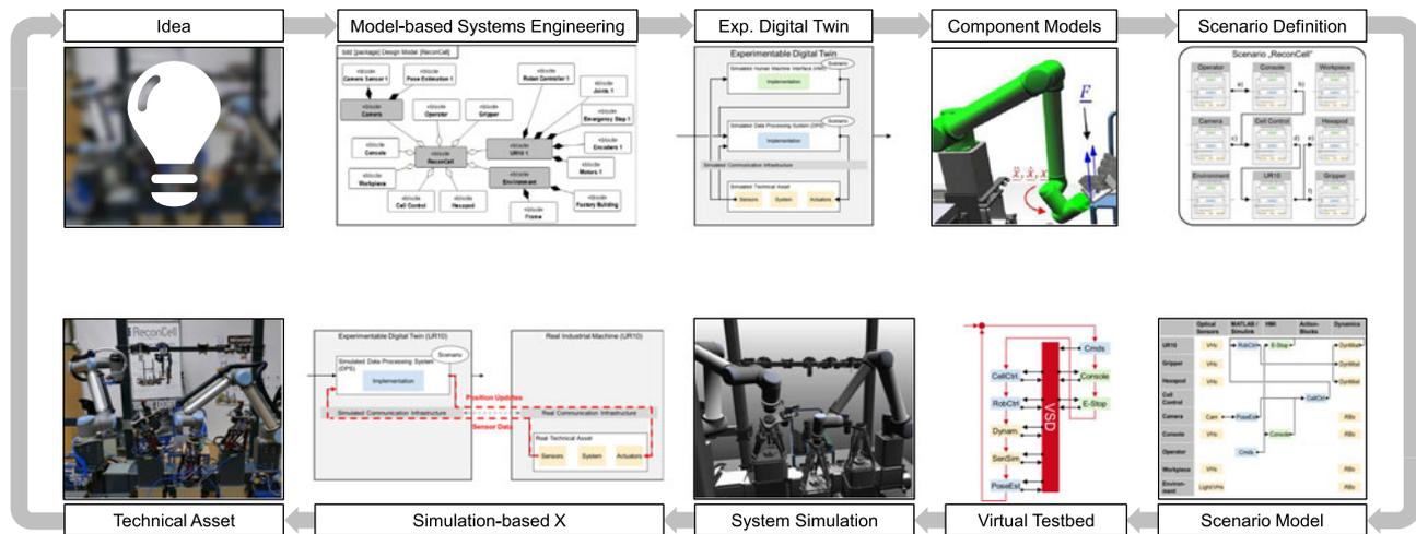
Fig. 16. Life-cycle spanning simulation-based systems engineering using EDTs.
