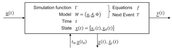
Fig. 7. Structure of the single components (blocks) of EDTs (based on [6]).
