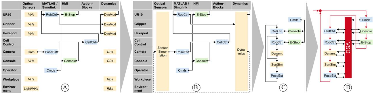
Fig. 9. Automatic model analysis process. a) EDT components and simulation algorithms with their explicitly modeled data flows and interactions. Columns are simulation functions, rows are EDTs, VHs = visible hulls, and RBs = rigid bodies. b) Automatic grouping by simulation functions, e.g., of sensor simulation and dynamics. c) Resulting simulation network, executed by the scheduler. d) Simulation results are routed via the VSD.
