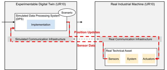
Fig. 13. Networking EDTs and their physical counterparts in SbC scenarios, here shown for a UR10 robot in the ReconCell.
