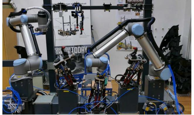
Fig. 12. Real setup of the virtual ReconCell shown in Fig. 1. All controllers are implemented via SbC.
