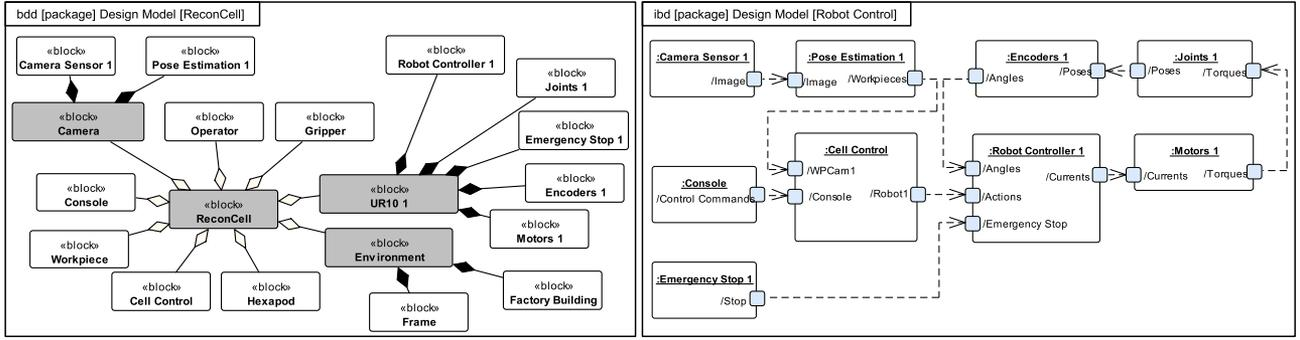
Fig. 8. Two (simplified) MBSE diagrams for the ReconCell use case.
