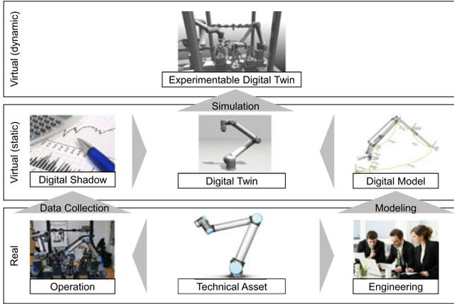
Fig. 3. Correlation of the Industry 4.0 terms “technical asset,” “digital shadow,” “digital twin,” and “EDT” (based on [18]).
