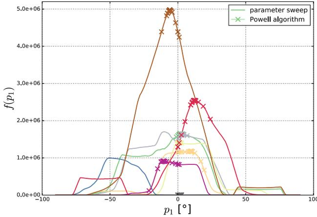
Fig. 11. Optimization results for (1). Lines show parameter sweeps  $f(p_i) \forall i$ . Crosses indicate evaluations by the Powell optimizer [23].
